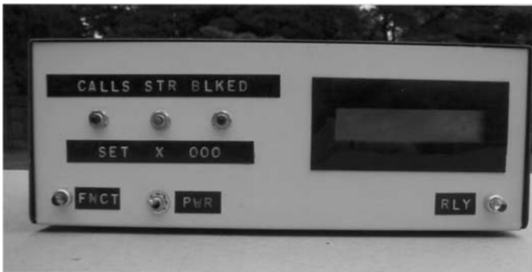
Figure 9-1 Caller ID project, as assembled.
