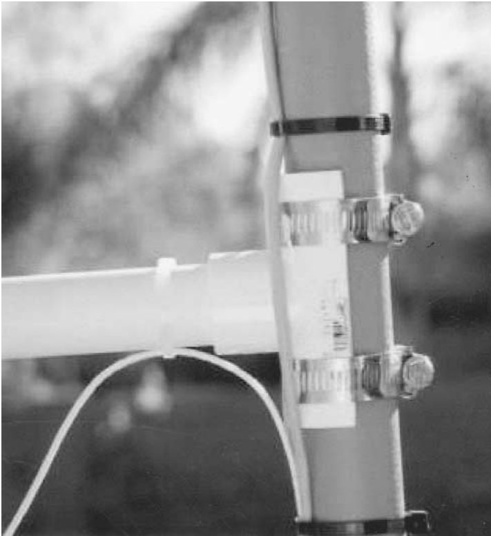
Figure 7-7 Securing the LSU to the mast.
